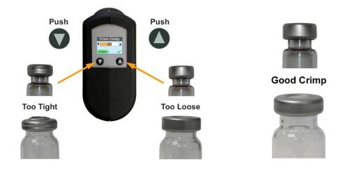
The cycle button must be held down until the crimp is complete. If the switch is released early the
